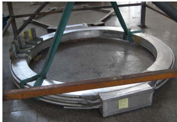
Fig. 9. Cold-mass assembly for large test coil at ICST.
