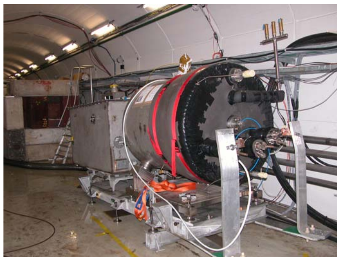
Fig. 3. MERIT experiment being installed in CERN TT2A tunnel.
