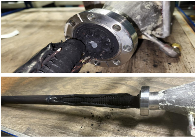
Figure 7: Site of arc on 10 of 12 pins in TBD
