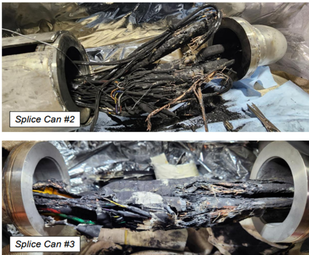
Figure 8: Wiring failure of 4 o'clock DX magnet
