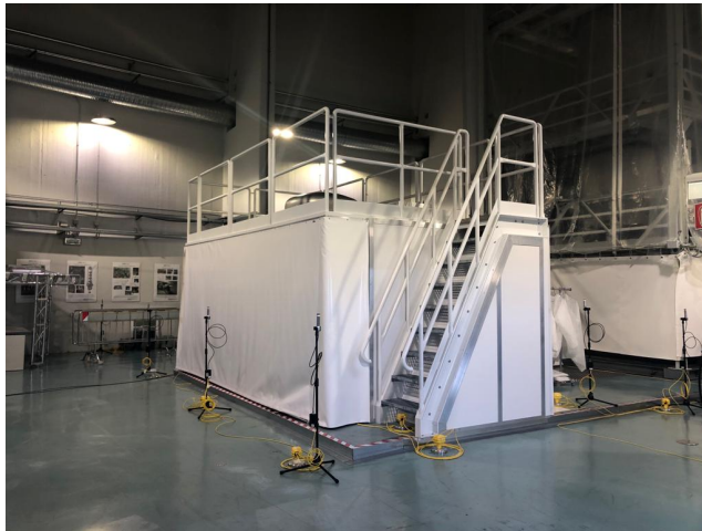
Figure 2.19: Seismometers and infra-sound microphones installed at the Advanced Virgo Plus site.
