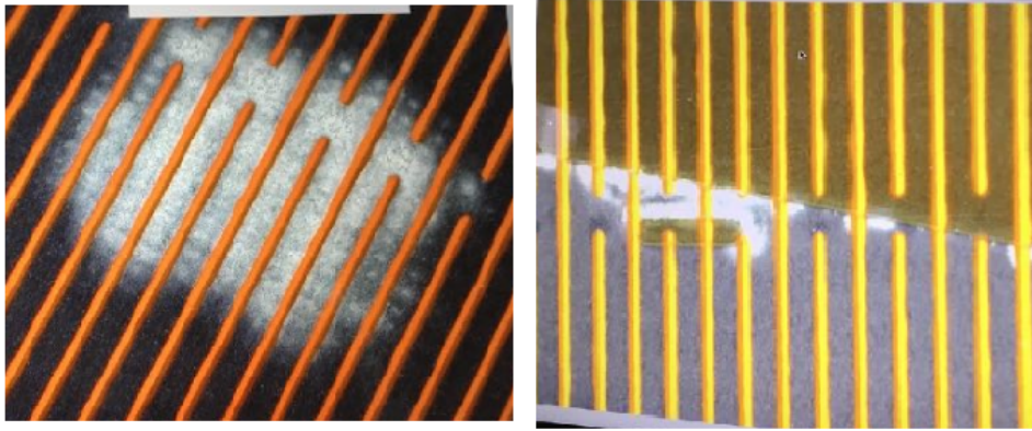
Figure 25. Pictures of a readout panel exposed to the equivalent dose of 1 month in ATLAS at high luminosity LHC conditions. Left: discharges residuals at strips interconnection zones. Right: discharges residuals close to the pyralux coverlay. Copyright 2020 CERN for the benefit of the ATLAS Collaboration. CC-BY-4.0 license.
