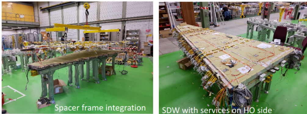
Figure 19. Two steps of the DW mechanical integration: a spacer frame while being mounted on a WE (left) and a fully equipped DW ready for cosmic ray test (right). Copyright 2020 CERN for the benefit of the ATLAS Collaboration. CC-BY-4.0 license.
