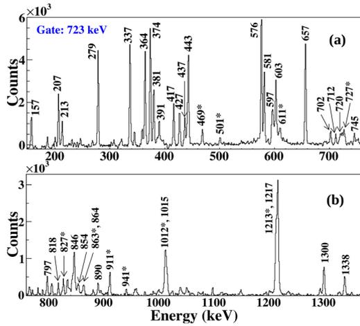
**Fig.1:** Coincidence spectra gated by 723 keV; (a) Lower energy (< 760 keV) part and (b) higher energy (>760 keV) part. Newly observed transitions are marked by ‘\*’.
