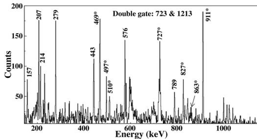
**Fig.2:** Double-gated spectrum with gates on 723 & 1213 keV, from the cube. The newly observed transitions are marked by ‘\*’.
