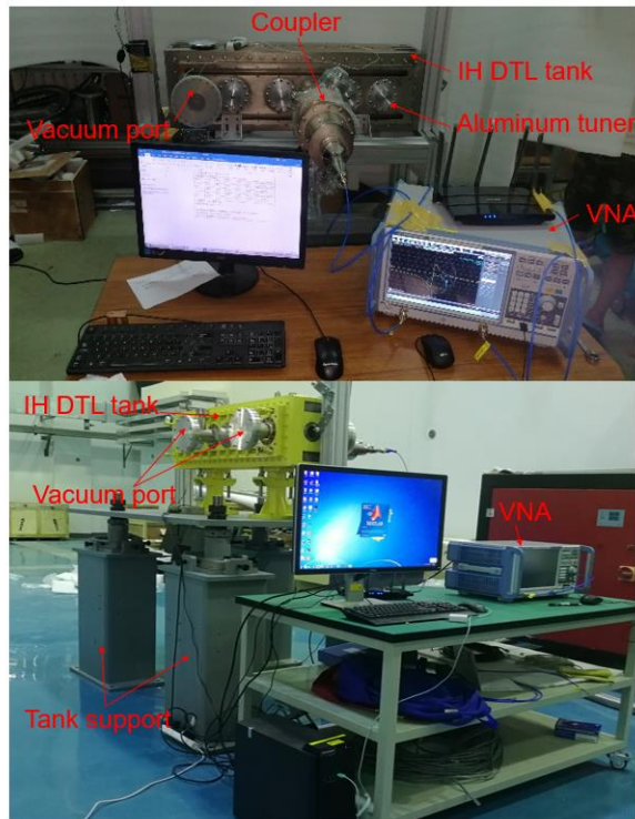
Figure 1: The low power test platform of the IH DTL (up: Tsinghua University, down: NIST).
