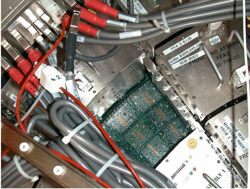
Figure 2.18: Partial view of drift chamber front-end electronics.
