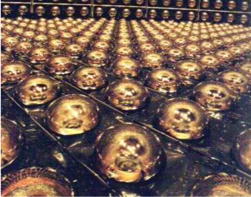
Figure 3.3: The Inner PMTs with black sheeting.
