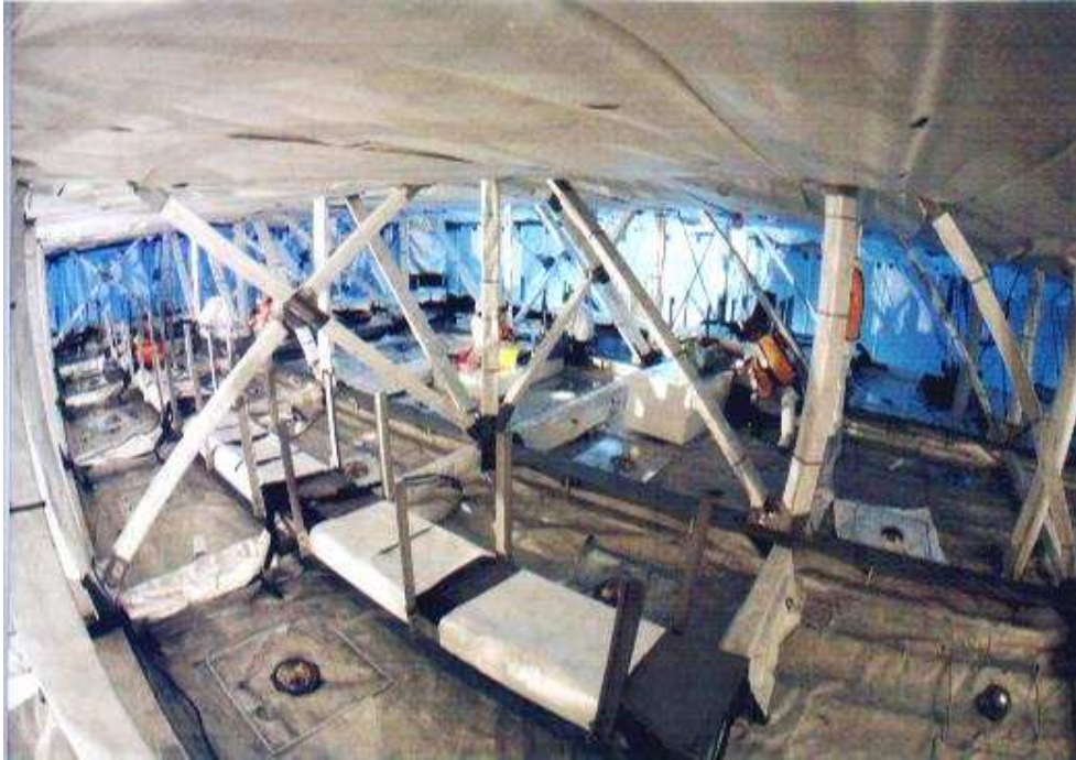
Figure 3.4: The OD PMTs on the top.
