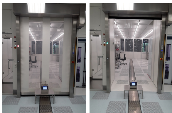
Figure 5: Closed (left) and opened (right) roll-up door with the particle counter placed in front of it in CR 1.
