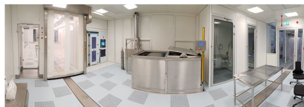
Figure 1: Fisheye perspective of CR 1 (ISO-6). In the middle part the US and C-rinse baths are shown, on the left: Personnel air lock, roll-up door and part of the HPR.
