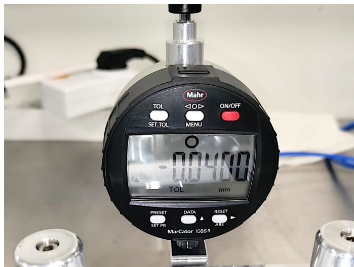
Figure 6.32: Typical calibration reading on the dial gauge for the thickness of the glue layer between the flex and the module.
