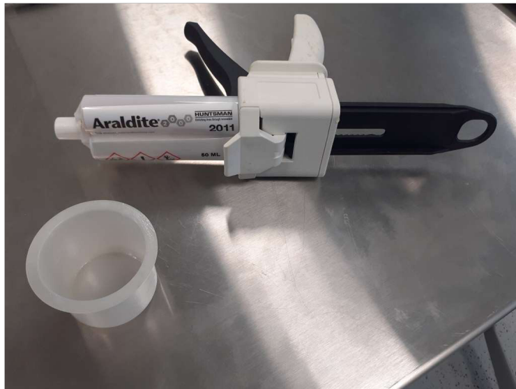
Figure 6.34: The caulking gun loaded with the Araldite 2011 adhesive container, and the disposable cup into which the glue mix was deposited.
