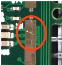
Figure 6.61: A scratched wirebond pad on the flex observed under the VHX-7000 microscope.
