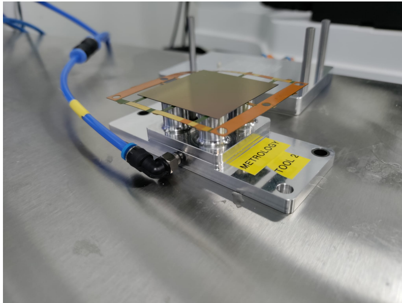
Figure 6.48: The pickup body was flipped over to reveal the bottom surface of the chips.
