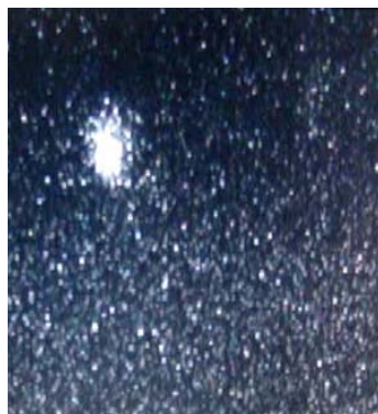
Fig. 2. Accelerated Neon beam spot on beam viewer
