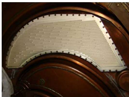
Fig. 4. Baffled of cryopanel placed in the dee
