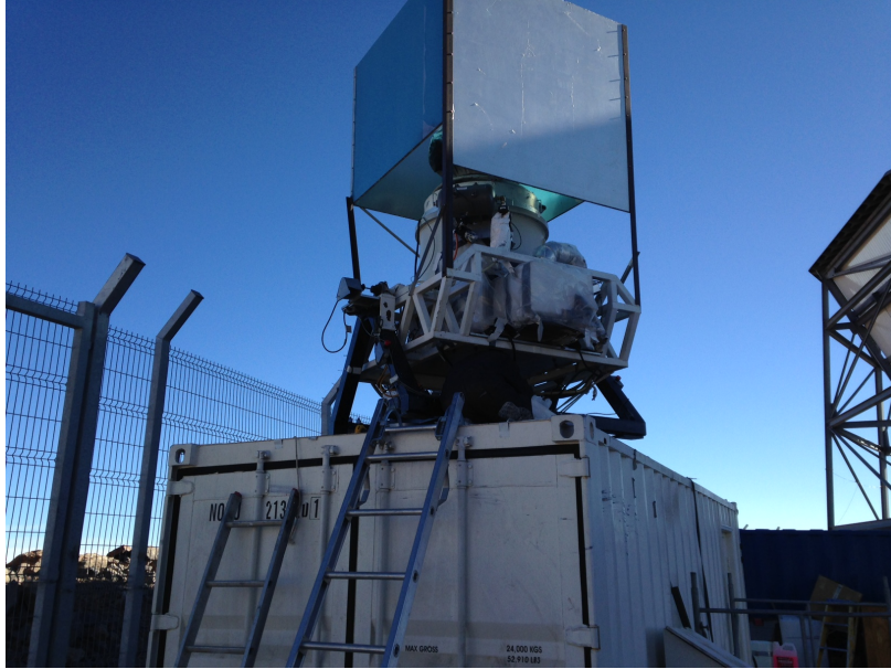
Figure 1.4: Picture of the ABS receiver during its final observing season in 2014. The blue structure is aluminum hexcell placed in a square mount to act as a reflective ground screen. The conical baffle and supporting shipping container can also be seen.
