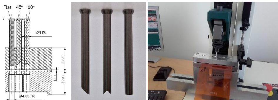
Figure 1. (a) Technical drawing of punching tool, (b) penetration probes 4 \times 100 DIN 9861 D, flat type, 90^\circ type and 45^\circ type and (c) punching tool installed in the universal test machine.
