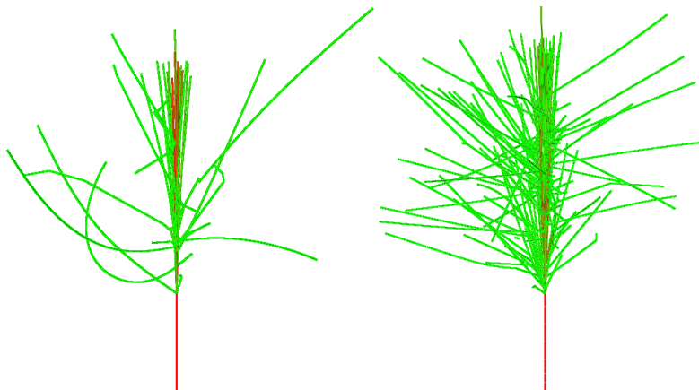
Figure 4.4: Qualitative comparison of particle shower sizes for a pion particle with low energy (left) and high energy (right) when entering the ATLAS calorimeter in a full (Geant4) simulation. The red line illustrates the initial pion particle. The green lines show secondary particles created by the detector simulation due to interaction of the pion with the ATLAS calorimeter detector material.
