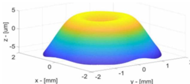
Figure 1: A measured SLB wavefront profile at the generator output, the beam propagates downwards along Z-.
