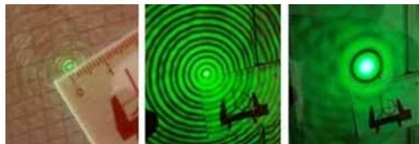
Figure 3: SLB images at 120 m, propagated outdoor, with different generator adjustments. The IC diameter varies from approximately 1 mm with a high number of rings (left) to 15 mm (right) with a low number of rings.
