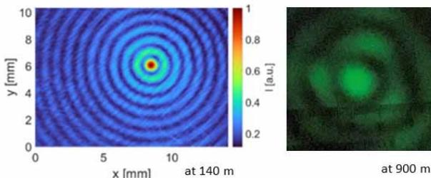
Figure 4: Real SLB measurement at a distance of 140 m from the generator, the optical intensity  $I$  is in arbitrary units (left). Picture of an SLB at 900 m distance from the generator, the IC is approximately 1 cm diameter (right).
