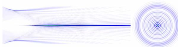
Figure 2: Simulated SLB longitudinal (left) and transverse (right) intensity distributions.
