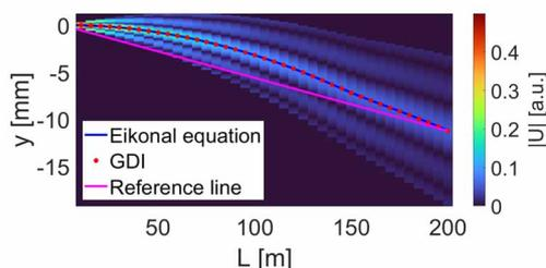
Figure 8: Longitudinal profile of the SLB field amplitude for temperature distribution based on measurement in the LHC tunnel at CERN.
