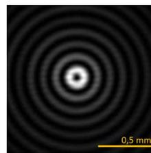
Figure 6: Intensity in the transverse plane of a real HSLB at 2 m from the generator.
