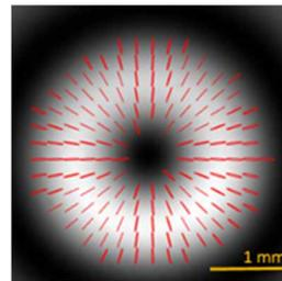
Figure 7: Image of a real HSLB at a distance of 50 m, cropped to the first light ring. The radial polarization in the transverse plane is represented in superposition.
