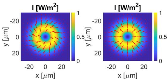
Figure 5: Input Beam with a spiral polarization. General case (left). Particular case with radial polarization (right).
