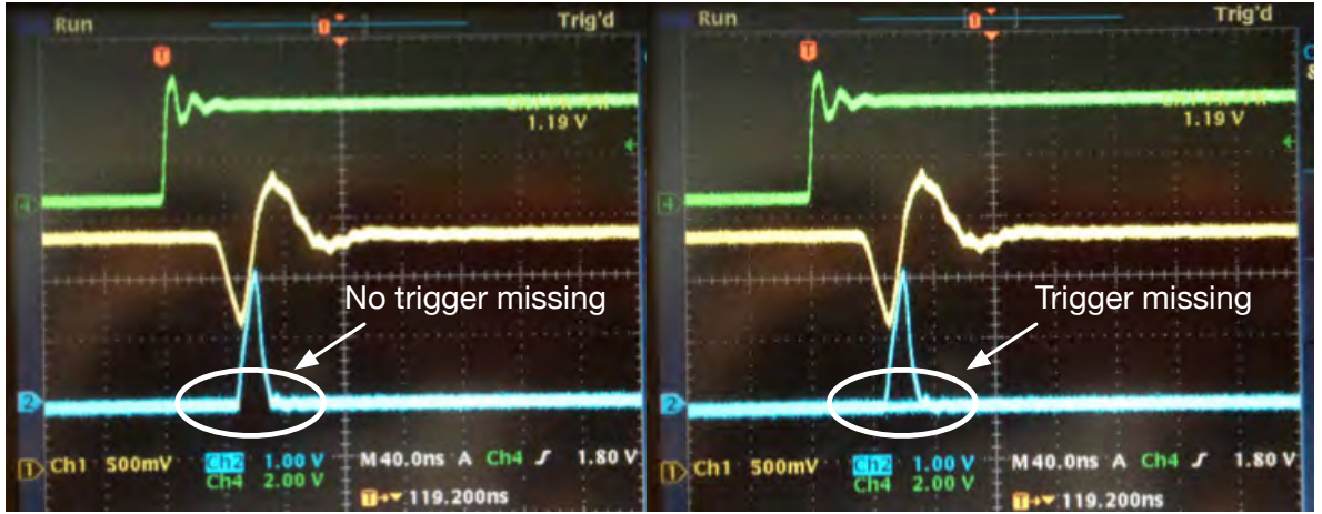
Figure 6.6: Comparison of the output of the non-delayed trigger with and without trigger missing. The left picture is the output of the non-delayed trigger without trigger missing. The right picture is the output of the non-delayed trigger with trigger missing. The green curve is the trigger signal from the signal generator. The yellow one is the output of the fast shaper. The blue one is the non-delayed trigger signal generated by chip itself.
