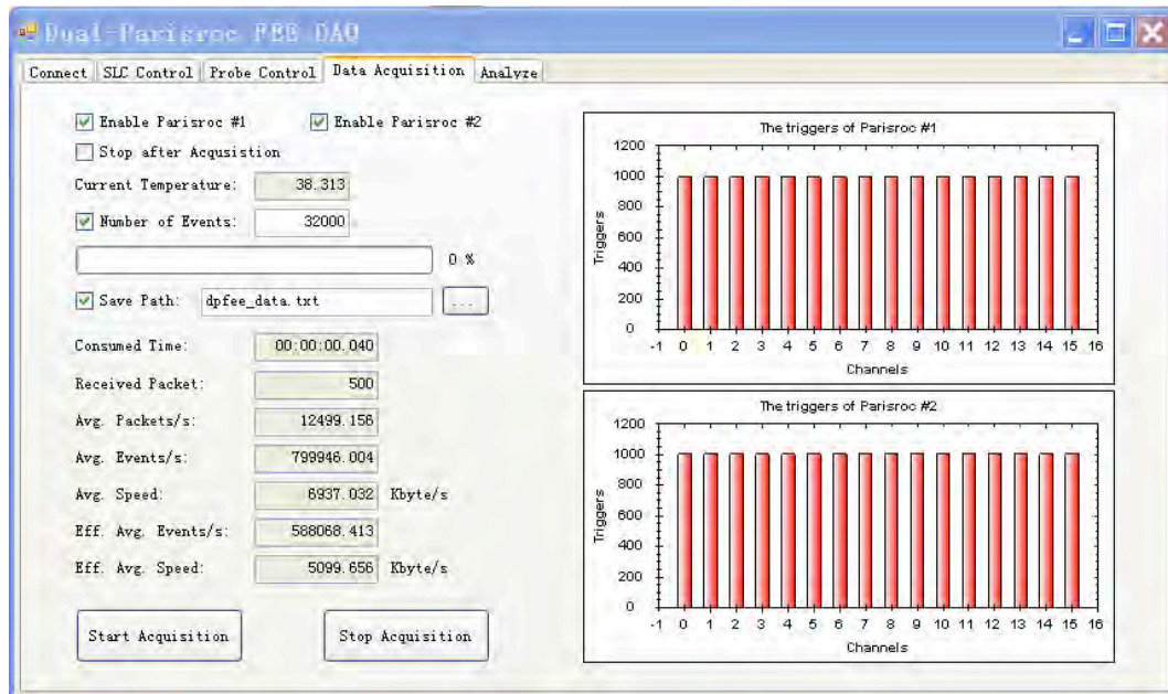
Figure 8.14: Maximum data output rate measured with the DAQ software
