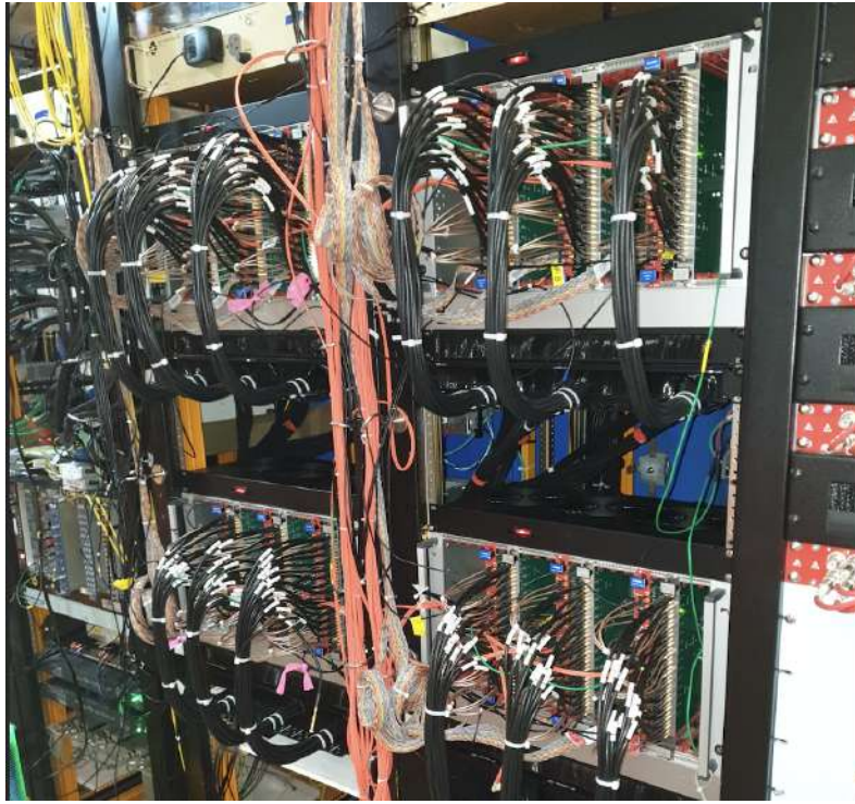
Figure 4.4: A picture of CAEN V1730B digitizer boards with the new WL-195N cables.
