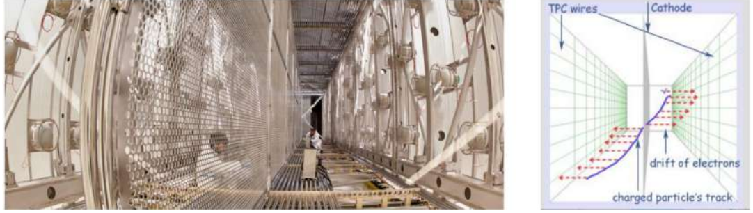
Figure 2.6: Picture (left) and scheme of one of the cryostat (right) [22, 30]
