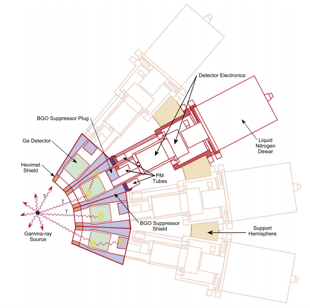
Fig. 5.5 A typical Gammasphere detector module [187]
