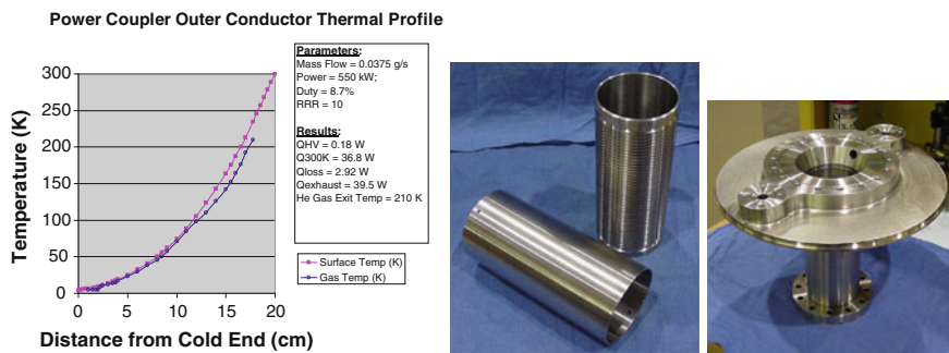
Fig. 6.16 He gas cooling passages ( right ) and FPC outer conductor assembly ( left ). The helium gas flow rate of 0.038 g/s produces an exhaust temperature of 210 K ( center )
