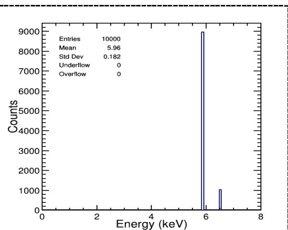
**Figure 10.** Energy peaks of  $^{55}\text{Mn}$  of 5.89 and 6.49 keV respectively obtained from simulation of gamma source in Ar-CO<sub>2</sub> (70-30) gas mixture using heed++.
