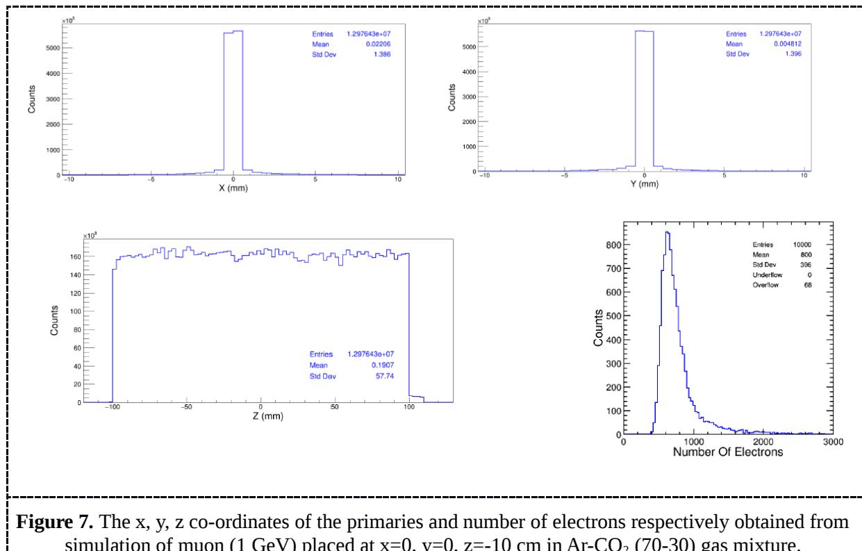
**Figure 7.** The x, y, z co-ordinates of the primaries and number of electrons respectively obtained from simulation of muon (1 GeV) placed at x=0, y=0, z=-10 cm in Ar-CO<sub>2</sub> (70-30) gas mixture.
