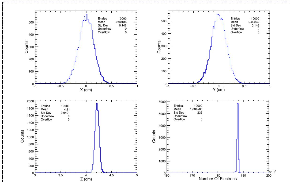
**Figure 6.** The x, y and z co-ordinates and number of electrons respectively obtained from simulation of  $^{241}\text{Am}$  (alpha of 5.6 MeV) in Ar-CO<sub>2</sub> (70-30) gas mixture.
