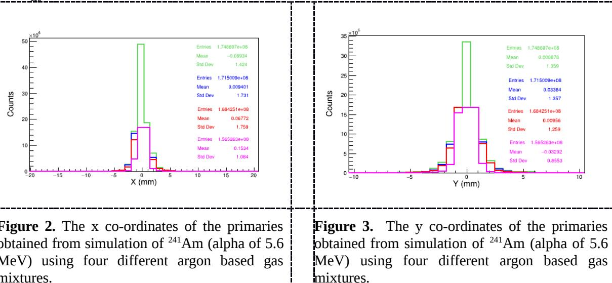
**Figure 2.** The x co-ordinates of the primaries obtained from simulation of  $^{241}\text{Am}$  (alpha of 5.6 MeV) using four different argon based gas mixtures.
