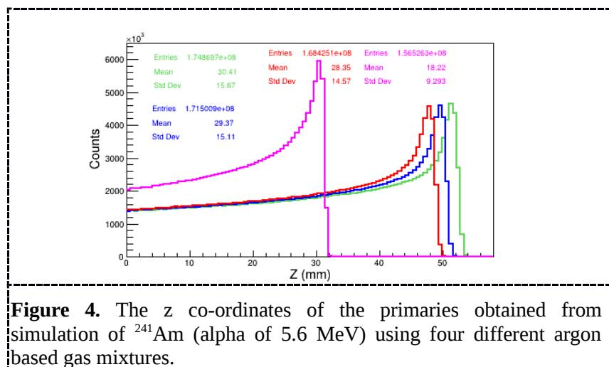
**Figure 4.** The z co-ordinates of the primaries obtained from simulation of  $^{241}\text{Am}$  (alpha of 5.6 MeV) using four different argon based gas mixtures.
