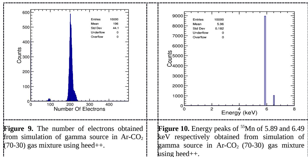
**Figure 9.** The number of electrons obtained from simulation of gamma source in Ar-CO<sub>2</sub> (70-30) gas mixture using heed++.
