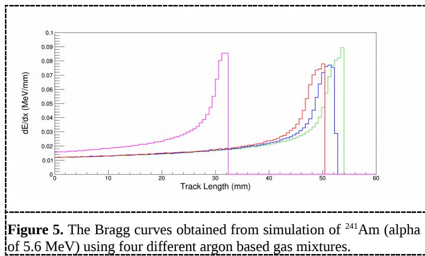
**Figure 5.** The Bragg curves obtained from simulation of  $^{241}\text{Am}$  (alpha of 5.6 MeV) using four different argon based gas mixtures.
