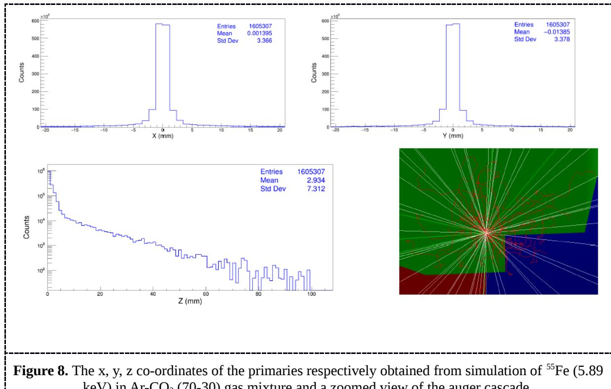
**Figure 8.** The x, y, z co-ordinates of the primaries respectively obtained from simulation of  $^{55}\text{Fe}$  (5.89 keV) in Ar-CO<sub>2</sub> (70-30) gas mixture and a zoomed view of the auger cascade.
