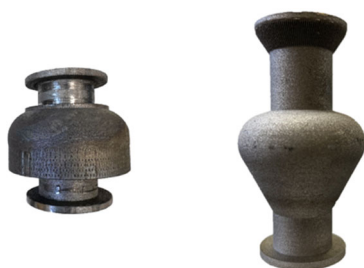
Figure 1: Seamless niobium cavities produced with LPBF process.
