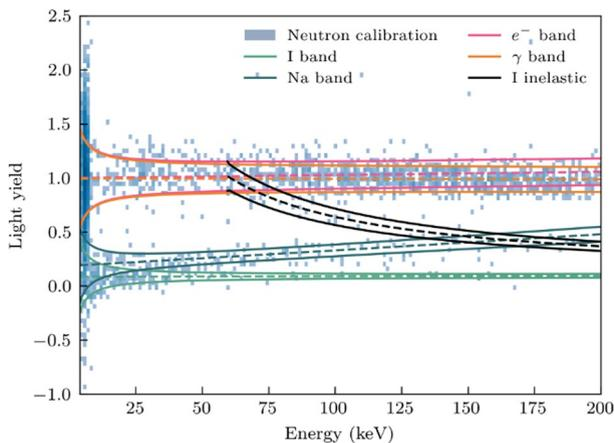
**Fig. 2** Light yield for events measured with a COSINUS detector prototype as a function of the energy measured in the phonon channel. An AmBe neutron source was used in the measurement to induce nuclear recoils. A parametric description of the LY bands and the corresponding energy spectra of the different event classes was fitted to the data, and  $e/\gamma$  and nuclear recoil bands are clearly separated. Figure from [9]
