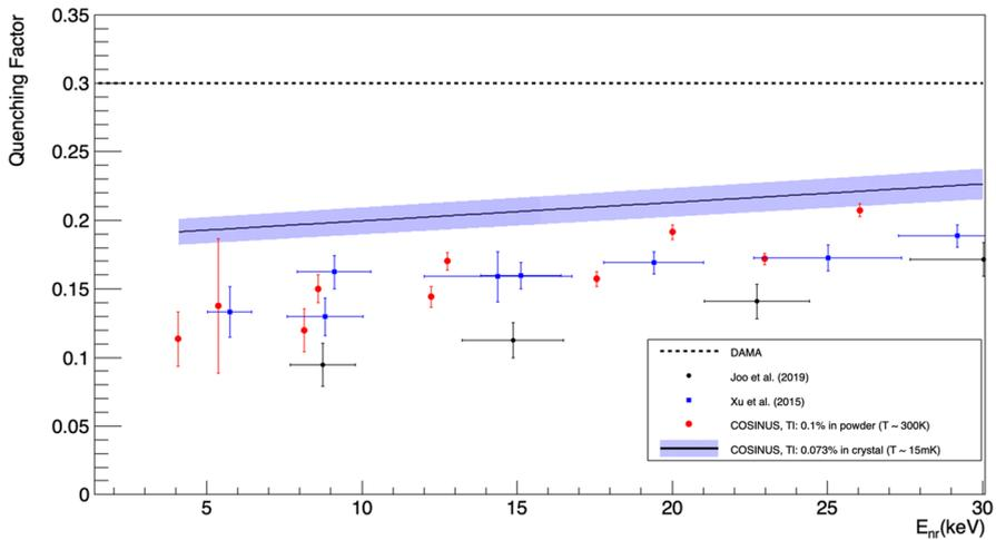
**Fig. 4** Na QFs measured with COSINUS NaI(Tl) crystals at room temperature at the TUNL facility (red dots), and at cryogenic temperature ([9], solid black line, with blue shaded uncertainty region). The constant QF assumed by DAMA (dashed black line) and results from [16] and [15] are shown for comparison
