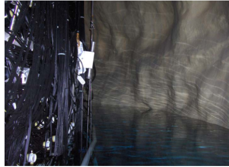
Figure 2: SNO+ cavity filled with water.
