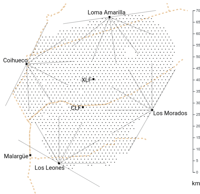
Figure 1. The layout of the Pierre Auger Observatory covering 3000 km 2 . Each small dot corresponds to a water-Cherenkov detector. Fluorescence detectors are located at Los Leones (LL), Coihueco (CO), Loma Amarilla (LA) and Los Morados (LM). The 30° azimuthal fields of view of the six telescopes at each site are shown by the radial lines emanating from them: the vertical reach of the telescopes extends to an elevation of 28.6°. Data are transmitted to the central laboratory, located at a campus in Malargüe, using a purpose-built communication network. The dashed lines show roads. Gaps in the layout of the array arise due to difficulties with landowners. Steerable lasers (see text) are located at the positions CLF and XLF.
