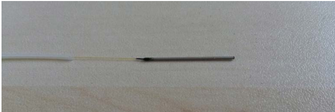
Figure 5. 4 FBG temperature sensor realized integrating a bare FBG inside the Al tube
