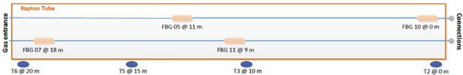
Figure 4. 11 Epoxy coated FBGs and CCS locations along the 20 m length Kapton tube
