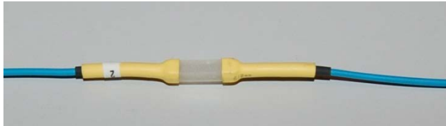
Figure 4. 2 PMMA coated FBG packaging for pigtails protection
