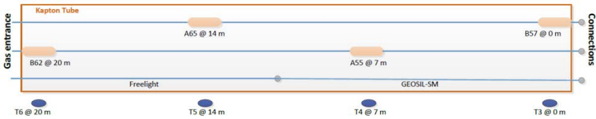
Figure 4. 5 PMMA and epoxy coated FBGs and CCS locations along the 20 m length Kapton tube
