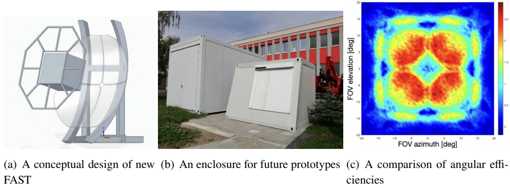
Figure 7: Developments for the FAST mini array. Optimization of telescope design is being discussed and some components are already produced for the next prototypes.
