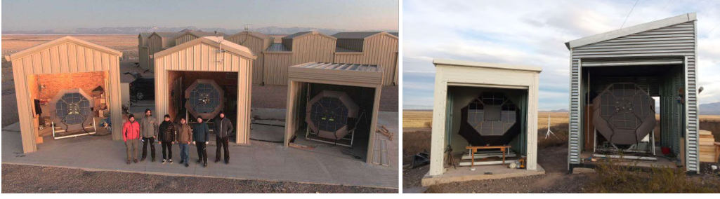
Figure 3: FAST prototypes in the Auger and TA site. Left: Three prototypes at TA are in operation. Right: Two prototypes at Auger. The second telescope (left in the picture) is not in operation yet [15].
