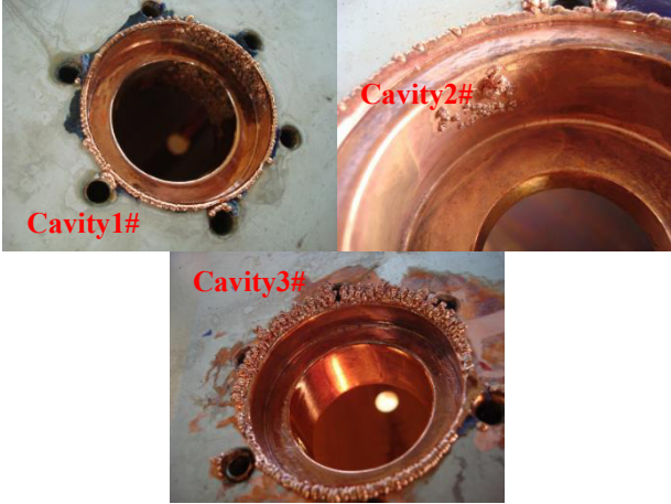
Figure 2: Electroplating of the first three cavities.
