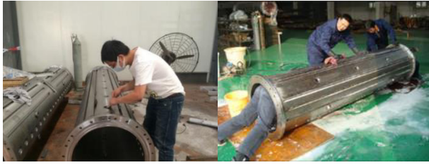
Figure 4: Surface acceptance and degreasing.
