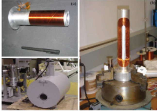
Figure 2.7: The FROST magnets clockwise from the top: the longitudinal holding magnet, the transverse holding magnet, and the polarizing magnet. Image source [43].
