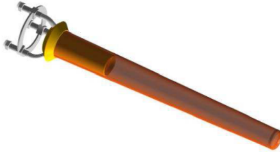
Figure 2.9: Target cell used during the g_{12} run period, placed 90 cm upstream of the CLAS center, and filled with liquid hydrogen. Image source [44].
