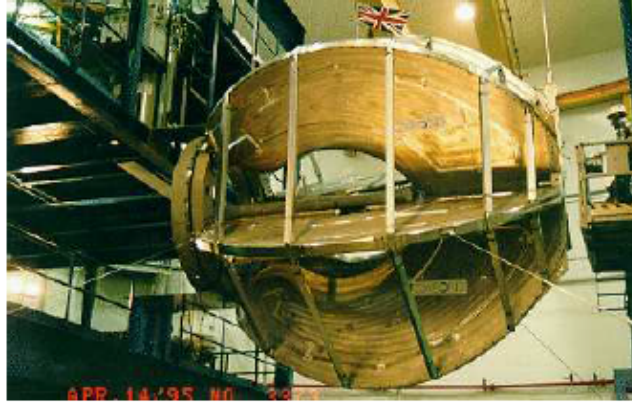
Figure 2.12: The CLAS torus coils in Hall B before installation of the rest of the detectors. Image source [41].
