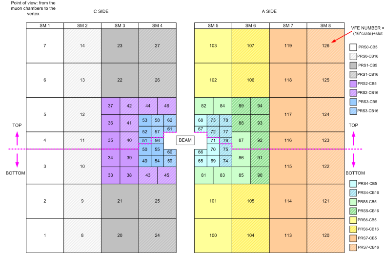
Figure 4.1: Disposition of the 100 SPD very front ends and their ID. The different sizes for the different parts of the sub-detector (inner, middle and outer) can be noted.
