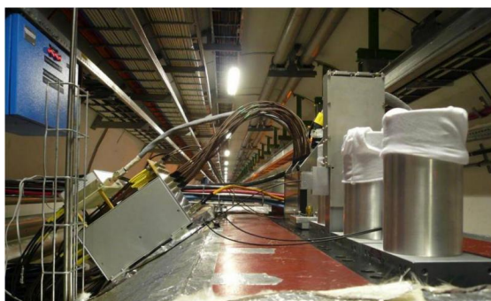
Figure 3.6: Picture of one of the LHCf detectors. Being the smallest detector at the LHC, its size is 80\text{ cm} \times 30\text{ cm} \times 10\text{ cm} .
