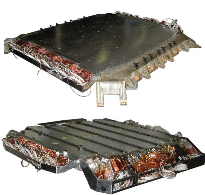
Figure 2.5: The completed upper and lower ToF before the final shielding. The scintillator paddles, the bent light guides and the PMT are exposed.
