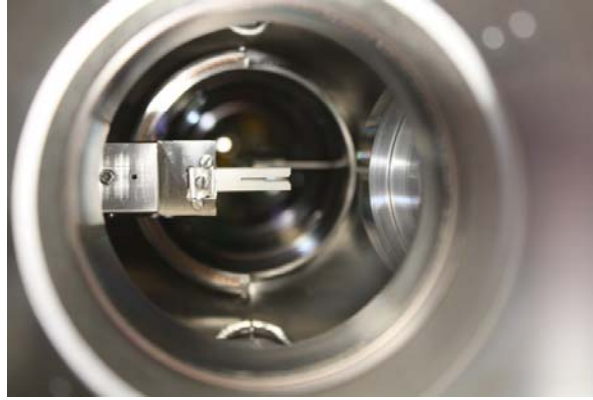
Figure 4: Dummy target in the vacuum chamber viewed from the downstream direction.
