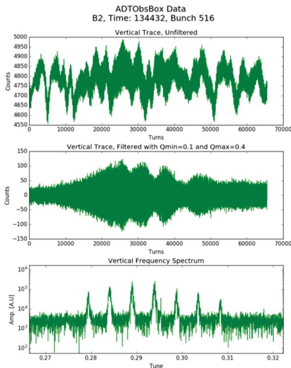
Figure 3: Single bunch coherent oscillation captured by manually triggering the ADTObsBox during the injection process. The top plot shows the unfiltered trace, the middle plot shows only the tune frequencies contribution to the signal with the FFT shown in the lowest plot.
