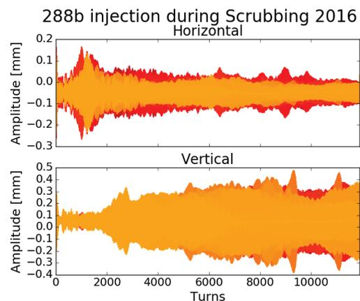
Figure 2: Injection oscillations from the only 288 bunch injection into the LHC in 2016. This injection triggered a beam dump due to transverse instabilities arising from the interaction with the electron cloud. The colour spectrum represents bunches at the beginning of the train (darker) towards bunches at the end of the train (lighter).
