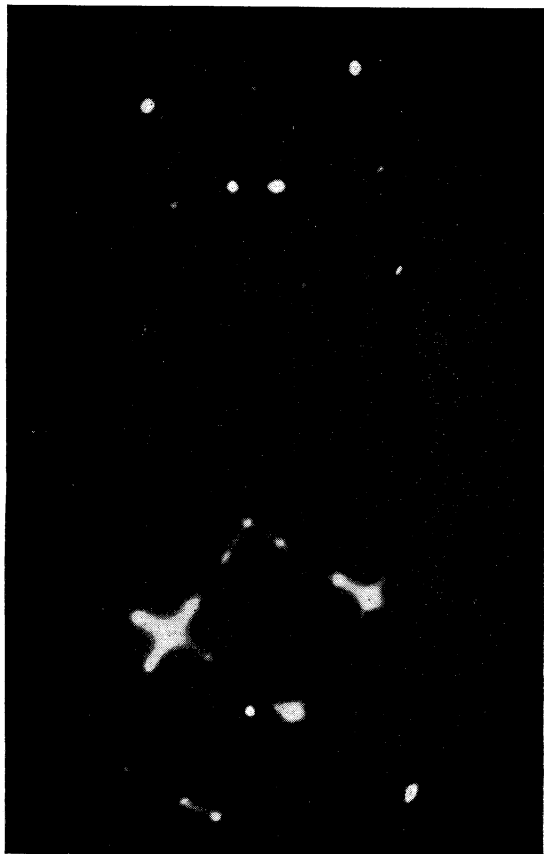
FIG. 2. (Top) Diffraction pattern characteristic of NbO-like structure can be seen as faint spots between more intense spots characteristic of clean Nb. (Bottom) Structure showing faceted structure on surface.
