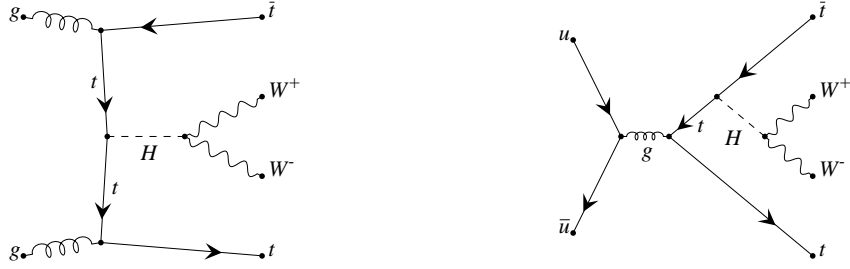
Figure 2: Some Feynman diagrams for the t\bar{t}H , H \rightarrow WW^{(*)} process. The dominant mechanism for t\bar{t}H production at LHC is the gluon fusion.
