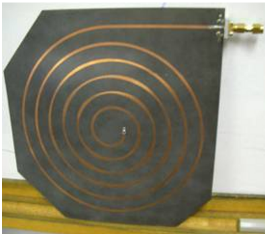
Figure 4.10: Prototype dedispersion filter. Photo by P. Roberts, ATNF.
