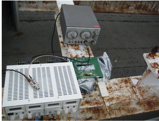
Figure 4.16: Analog pulse generator set up on the roof of the ATCA control building. ( From back to front ) The waveform generator (grey box) drives the ECL gate (on the green board). The output of the ECL gate passes through a 1–2 GHz bandpass filter (silver rectangle) and a signal amplifier (small square box). The large white box to the left is the power supply.
