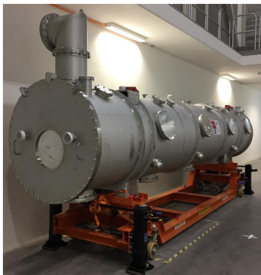
Figure 3: Cryomodule for installation tests at ESS.
