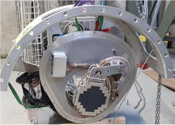
Figure 7. The radiative decay counter fully integrated in the MEGII apparatus.
