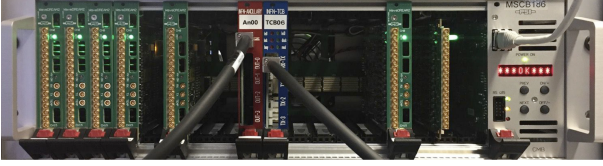
Figure 9. A TDAQ crate equipped with some WaveDREAM boards, a Trigger Concentrator board and an Ancillary board.
