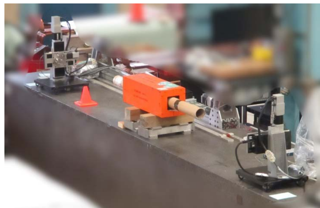
Fig.1. SSW system measuring a quadrupole magnet.
