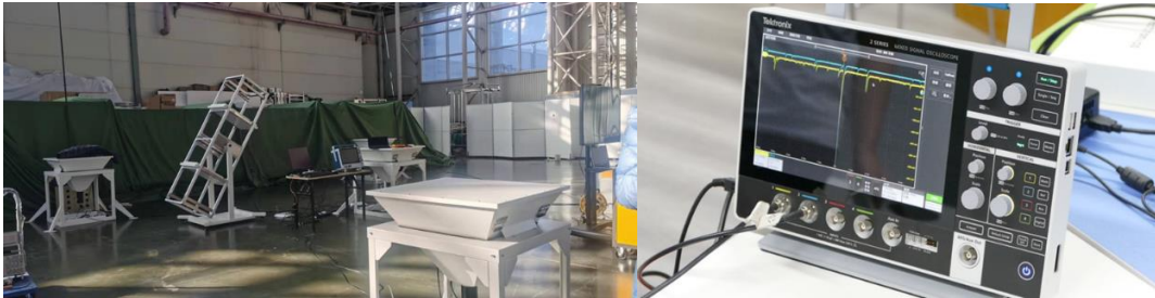
Figure 1: The cosmic ray observation array unit and the muon telescope.
