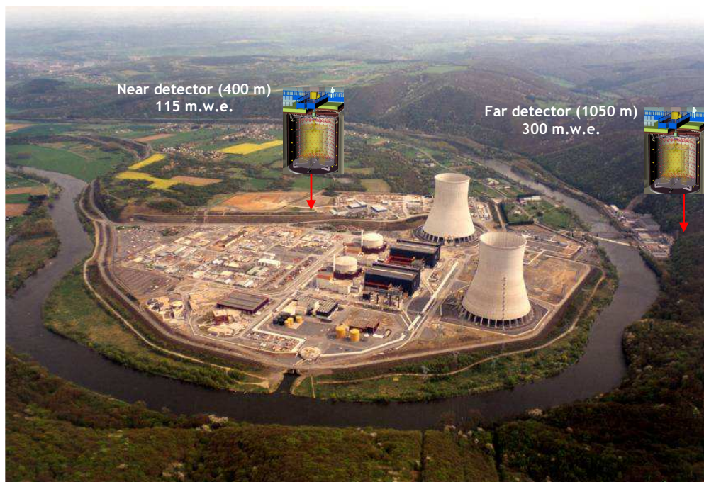
Figure 1. Location of the two Double Chooz detectors in the Chooz-B nuclear power plant.
