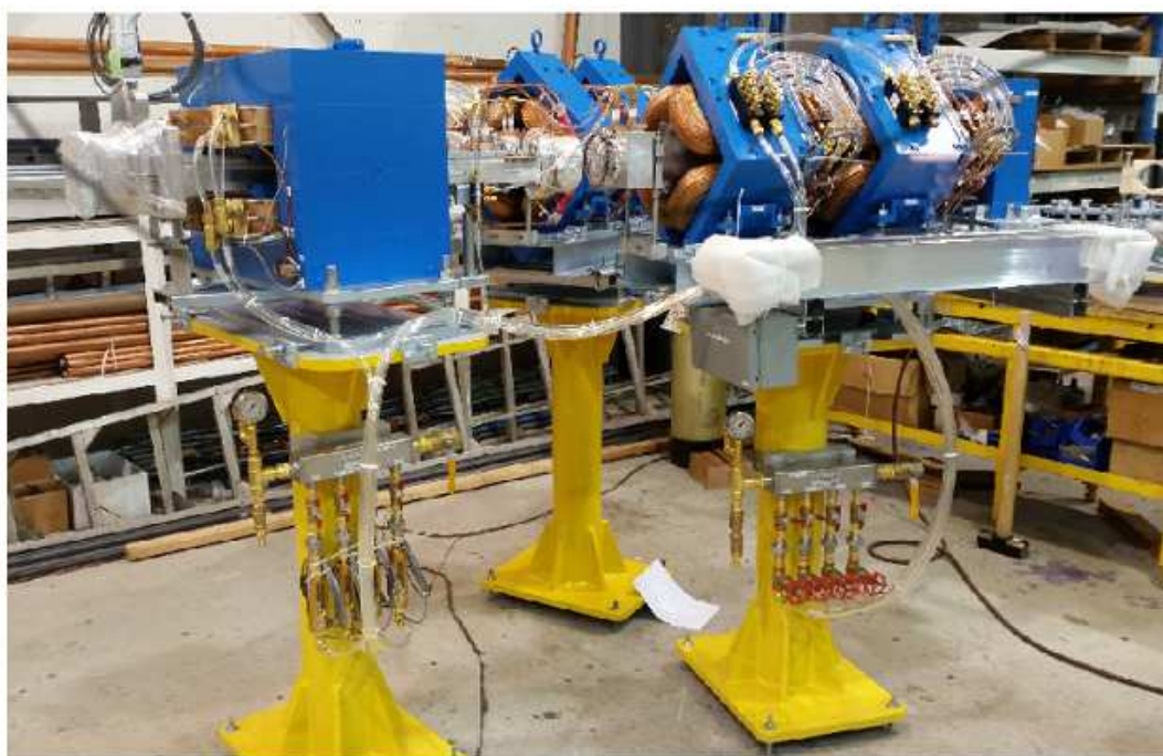
Figure 2. A Y-line belonging to the Sofia cyclotron.
