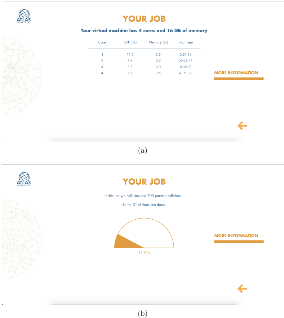
Figure 8.3: Screenshots of new features added to the ATLAS@Home graphical interface: (a) table with run time, CPU and memory information for the individual virtual machine cores running the task, and (b) progress bar indicating the task completion rate.
