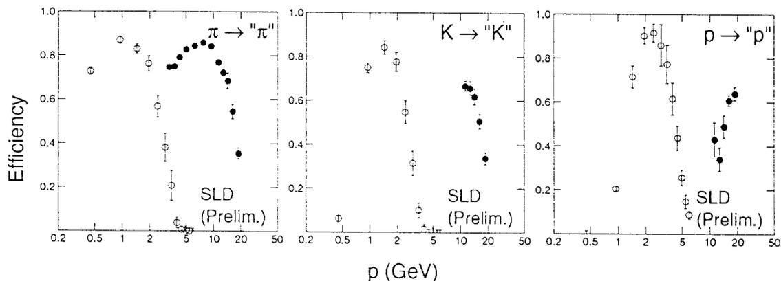
Figure 1: Identification efficiencies for charged  $\pi^\pm$ ,  $K^\pm$ , and  $p/\bar{p}$  for the SLD CRID, with systematic errors. The open circles are for the liquid radiators; the closed circles are the gas.
