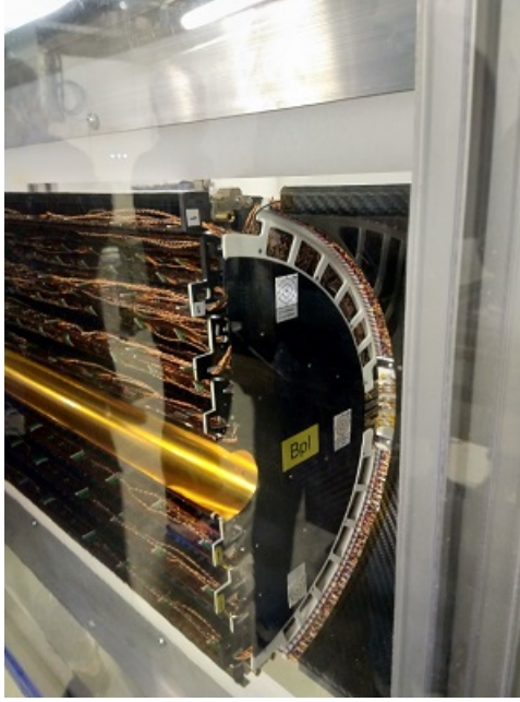
Figure 3.7: One half of the barrel BPIX detector with its four pixel layers. Photo taken during the long shutdown between the LHC data taking Run 2 and Run 3 where the pixel detector was extracted for maintenance in January of 2019.
