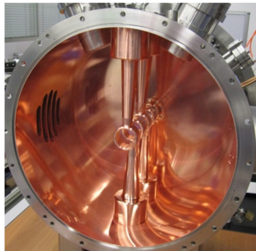
Figure 1: Detail of the interior of a buncher cavity.
