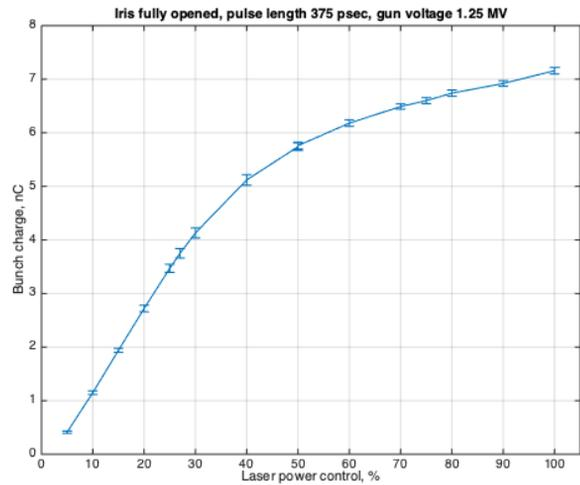
Figure 7: Dependence of the bunch charge vs laser power. Gun voltage is 1.25 MV, cathode recess is -10.5 mm, laser pulse length is 375 psec, laser spot diameter is 6 mm.
