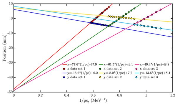
Figure 5: Horizontal and vertical position of the beam center as function of the inverse beam rigidity for three different trim sets. The intercept values and distance from the gun to profile monitor (4.27 m) give horizontal angle of  $-11.1 \pm 0.1$  mrad and vertical angle of  $+1.6 \pm 0.2$  mrad.
