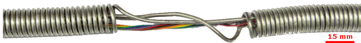
Figure 6.10: 4-K probe RF line shock coils. Note the right hand coil transitions to a straight segment transversing the center of the left coil, and the left coil transitions to a straight section transversing the center of the right coil. Each RF line acts as an independent spring and shock absorber while supporting the MSA sample. The RF cables are the greatest source of conducted heat from room temperature to the liquid helium bath, and the coiled sections add considerably to the length (and thus reduce the thermal conduction) of the RF cables.
