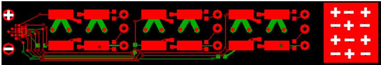
Figure 6.3: Board layout for in-line filter. Full layout file available at [105].
