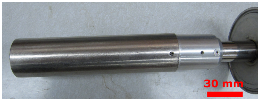
Figure 6.14: 4-K probe magnetic shield.
