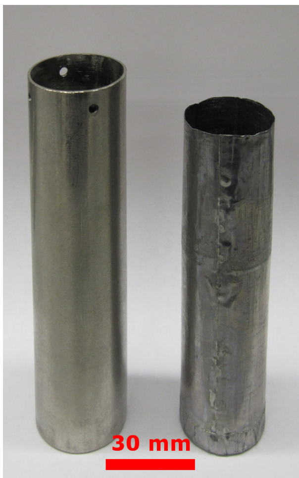
Figure 6.16: 4-K probe magnetic shield and lead liner. The lead liner tends to “lock in” the static magnetic field present when it cools through T_c , but greatly attenuates and AC fields (for example, 60 Hz) inside the liner. Note the continuously soldered joints. The author has the manual skills to achieve soldered joints on 0.2-mm lead foil, but has insufficient writing skills to impart the skills with verbiage. We recommend practice, patience, and a hot-air solder re-work station.
