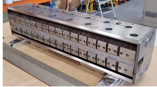
Figure 1: The SMH58 septum magnet out of the vacuum tank (length x width x thickness of the septum blade [mm]: 803 x 25 x 3).
