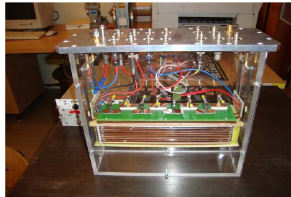
Fig. 2 GEM-TPC prototype in laboratory measurements in Bratislava
