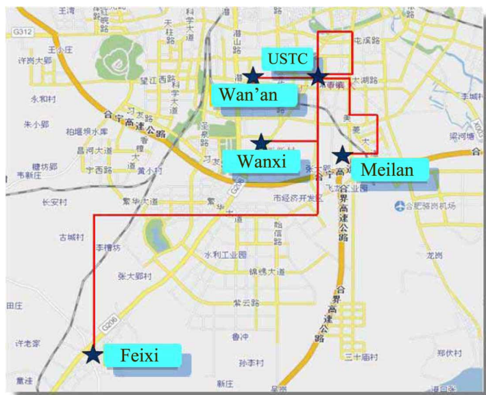
Fig. 1. Metropolitan all-pass quantum communication network constitutes 4 nodes including USTC', Wan'an, Meilan, and Wanxi. A circle link of 10 km goes back USTC through underground optic fiber cable, which is used to simulate a separately remote node USTC'. An additional node in Feixi county (finally moved to Tongcheng city) that is about 60 km fiber distance (130 km fiber distance) far from USTC' site in Hefei city, is further connected to achieve an inter-city QKD network, when the USTC' node serves as a trusted relay.
